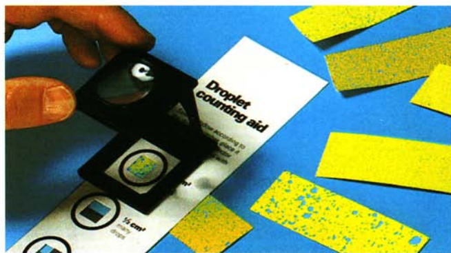
Linen tester lens together with the droplet counting aid card on an exposed collector paper.
